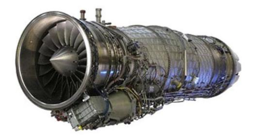
The jet engine forces air backwards with a maximum force of 90 000 Newtons (N). **Law 3** then says that there must an equal and opposite forward force, called thrust, of 90 000 N.
